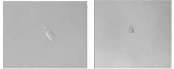
(c) Around 470\ \mu\text{m} in length inside 500^\circ lens (d) Around 270\ \mu\text{m} in 250^\circ lens
